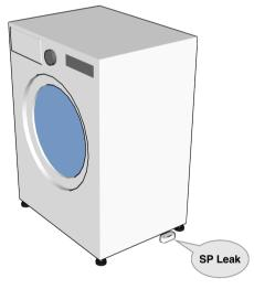
4. Install the sensor in the place of a potential leak by securing it to the floor with adhesive tape. It should be borne in mind that the reception area of the radio signal may be worse away from the windows.
