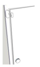
4. Install the main unit on the control doorway and magnetic unit on the door. Make sure that when closing the door, the units do not touch each other, while the distance between them does not exceed 5 mm.
