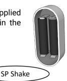
4. Install the sensor on the control object or inside the container by attaching it with ties or adhesive tape.
